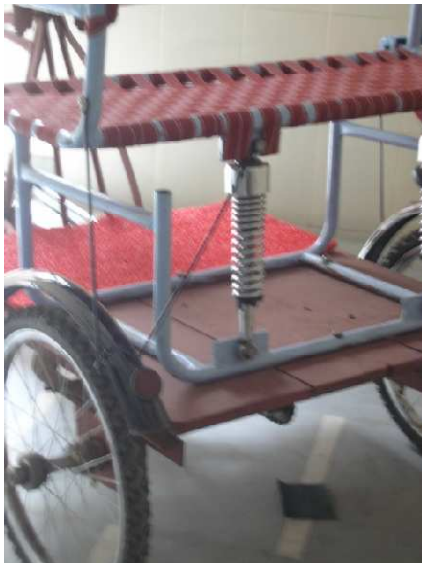
Figure 3 : Fazilka Femto Ecocab with Suspension System
